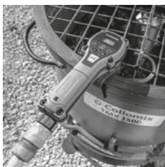
Mounting on a mixer drum
